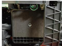
5. Reinstall the air cleaner cap. Reassemble the outer cover on the unit.
